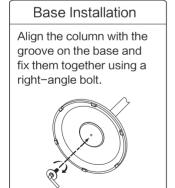
Considerate Hint: Remove ①②parts from the component before performing installation.
