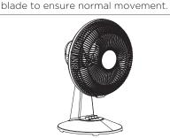
6. Install the Front grille by placing the Front Grille over the Rear Grille and using both hands to squeeze the Grilles until a clicking noise is heard. Ensure that the Front Grille is over-top of the Rear Grille in all locations.
