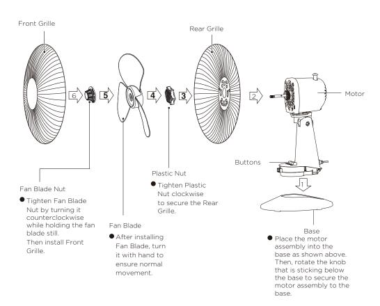
Rear Grille, Fan Blade, and Front Grille Installation
