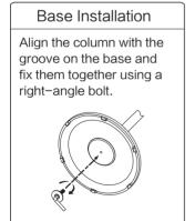
Considerate Hint: Remove ①②parts from the component before performing installation.
